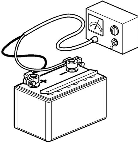
If the battery has discharged it must be charged. If the boat has not been used for some time charge the battery and then trickle charge it (see manufacturer's recommendations). A poorly charged battery will be damaged and may burst in cold weather.
