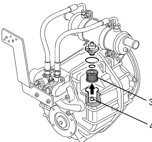
6. Install the new filter (3) in the filter housing.
